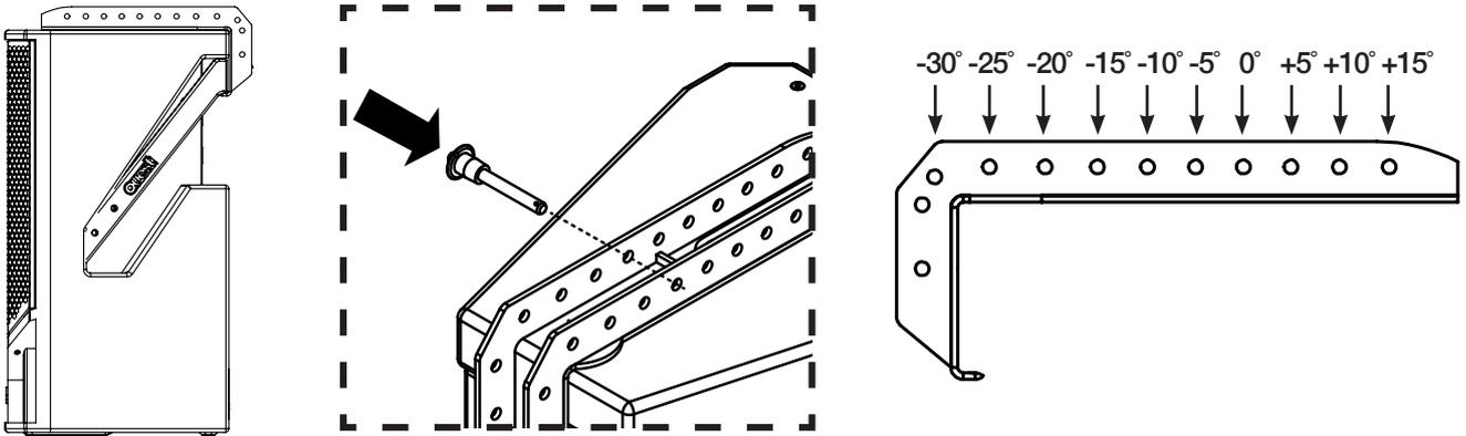
A suitably rated shackle is necessary to use the T-Spine in most applications (a ball lock quick-pin is included with the t-Spine).
