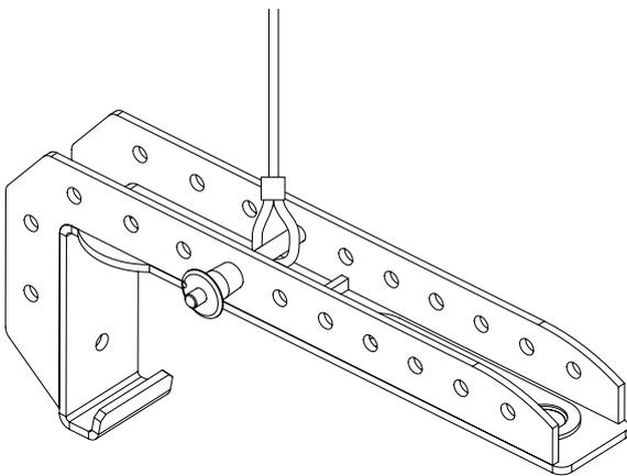
A safety wire connected to the speaker casing is recommended. Please consult local rigging regulations.
