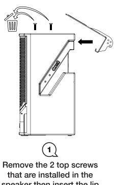
that are installed in the speaker then insert the lip of the Spine to grab the casing handle.
