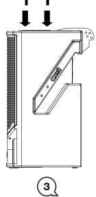
Bolt in and secure the Spine (using fastener securing compound) onto the speaker with the 2 x M10 bolts included.
