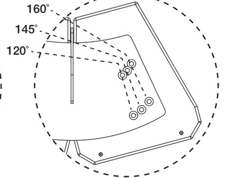
3. Bolt in the M10 x 35mm counter sunk screws included in the kit to lock the position to the required coverage angle.
